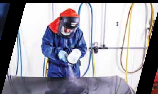
STEP 3: Clean area thoroughly and apply clear coat.
