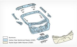
**Aluminum** — is a fast-growing rival of steel and is now used more often in modern vehicles because it's light and reduces the vehicle's weight. Aluminum is lighter than steel and by weight stronger as well. Parts of a vehicle that are typically made from aluminum include various engine components and wheels, but can also be found in some vehicle hoods such as the 2017-2022 Prius Prime hood.
