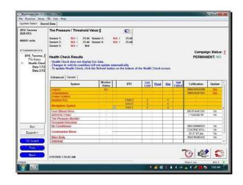
health check, you could miss the fact that the impact may have also affected the front-end ADAS systems even though that damage was not visible.<sup>2</sup>
